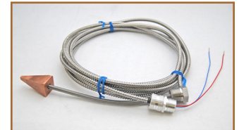
Figure 1. The WORM Flexible Temperature Sensors created for this installation include a specially-designed copper head that allowed the sensor to touch the bearings and draw heat to get the most accurate temperature readings possible.
