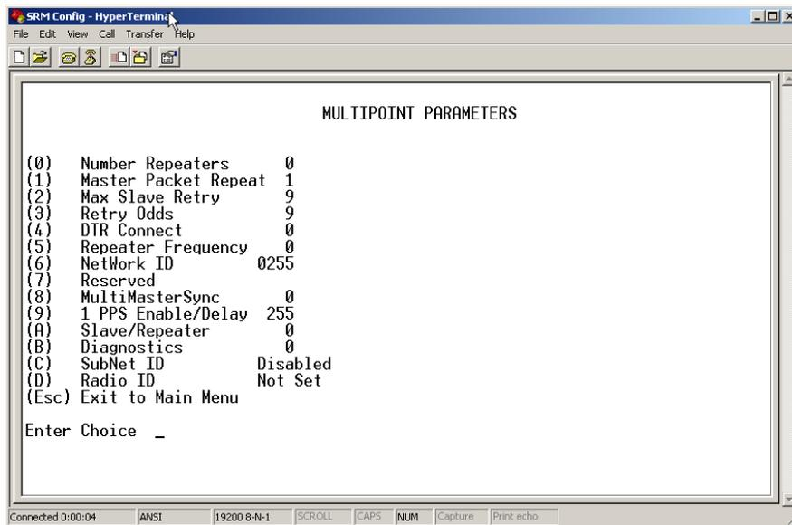
In a multi-point network, it is critical to know how many radio modems are being used as repeaters. Any radio modem that is used as a repeater essentially becomes a master to the remotes and other repeaters to which it is communicating. Therefore, the user must first identify how many repeaters are connected to the master by assigning a value in parameter
