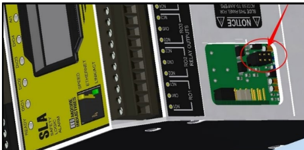
Figure 4.11 Relay 4 jumper moved to the stowed position, changing relay to a process relay.
