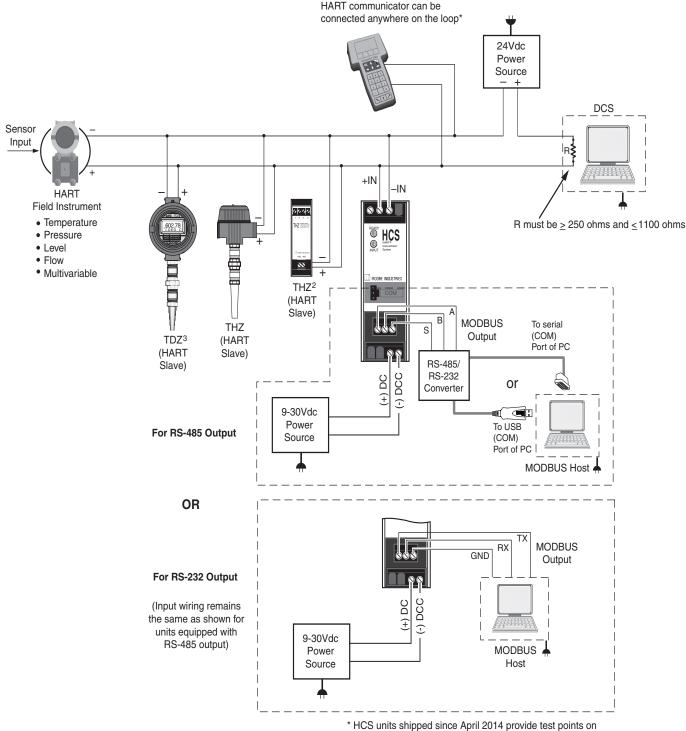
the +IN & -IN terminals for connecting a HART communicator
