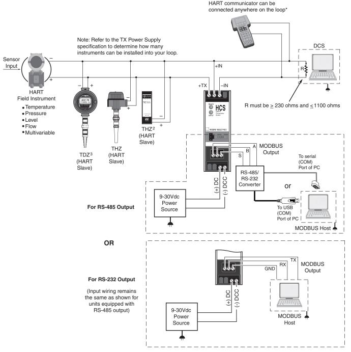
\* HCS units shipped since April 2014 provide test points on the +IN & -IN terminals for connecting a HART communicator
