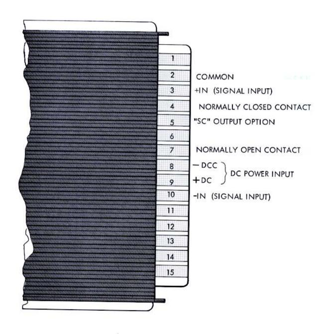
Figure 2-3. Electrical Connections For Plug-In Units
