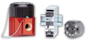
The SIY combines smart digital technology with advanced analog operation to deliver superior reliability, accuracy, and ease of use. The highly versatile SIY programs to accept a wide range of current or voltage inputs. It outputs an isolated, proportional, 4-20mA signal. As a flexible analog/digital hybrid, this 2-wire (loop-powered) transmitter programs in seconds with easy to use free software to handle a wide range of important signal interface applications.
