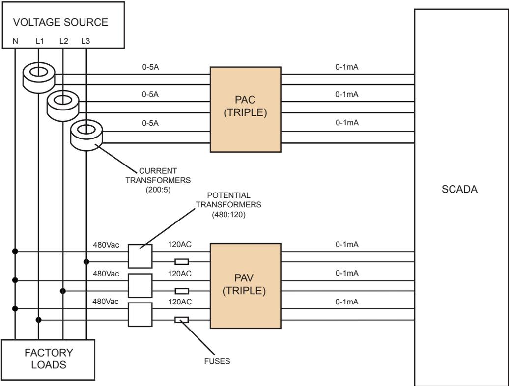
Figure 3. The PAC and PAV can be used to activate an alarm to avoid damage to voltage sensitive equipment.
