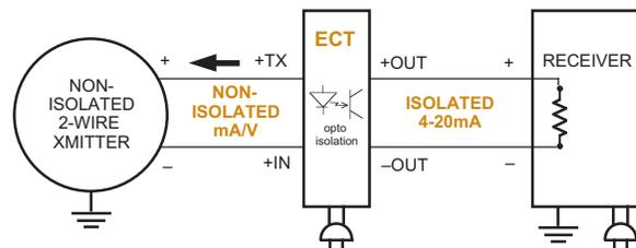
**Figure 11.** The ECT takes one process input and delivers two completely isolated signal outputs.
