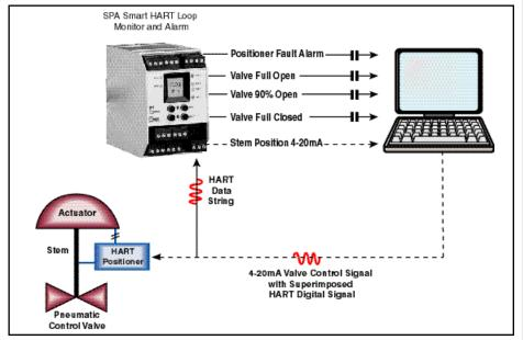
HART communicating valve positioners used in conjunction with HART loop monitors provide a reliable and cost-effective ESD strategy for emergency shutdown valves.
