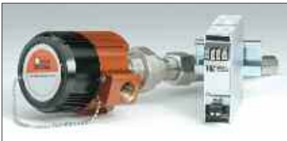
Figure 1: If an instrument meets design safety requirements, it can probably pass ATEX. The THZ2 and TDZ2 family of HART Temperature and Signal Transmitters from Moore Industries have acquired ATEX, cFMus (US/Canada), IECEx, CSA, and ANZEx (Australia) approvals for intrinsically-safe, non-incendive, and explosion-proof applications for Zones 0, 1 & 2.
