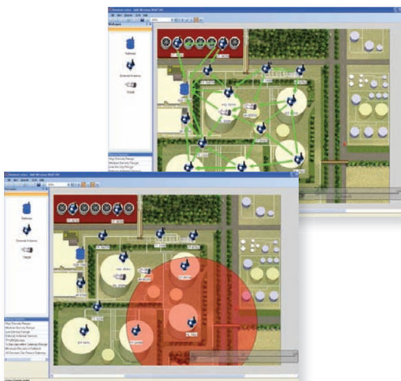
Figure 4: WirelessHART device networks can be designed easily with this visual network manager
