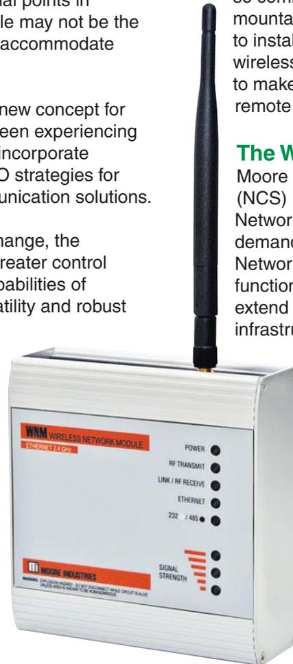
This bi-directional, spread spectrum wireless module employs Spread Spectrum Frequency Hopping technology, 128-bit AES (Advanced Encryption Standard) encryption, 32-bit CRC (Cyclic Redundancy Check) error protection and ARQ (Automatic Resend Query) to provide robust and secure, communications. The Spread Spectrum Frequency Hopping technique ensures reliable, noise and interference immune, license-free wireless communications.
