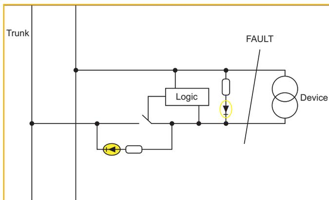
Tests by Evaluation International, an independent instrumentation testing and evaluation service, confirm the advantages of the fold-back technique: When a spur is short-circuited, segment voltage actually increases, because the device coupler removes the shorted device from the segment. This means multiple short circuits on a segment cannot deprive other instruments of power
