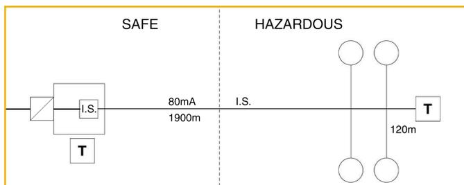
This optimistically could only power four fieldbus devices which typically take 15-26mA each. The Entity barrier concept is safe, but its low-power limitations and engineering requirements effectively eliminates many of the benefits of using bus technology.
