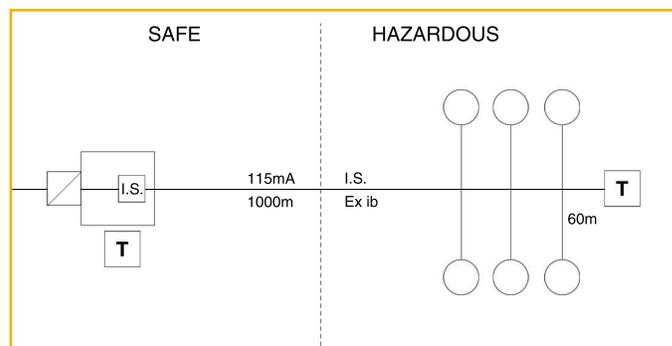
The FISCO concept considers the entire circuit of the fieldbus segment. This solution requires that each part of the system including devices, cables and power conditioners are FISCO certified and that FISCO design and installation rules are strictly followed (IEC60079-27).
