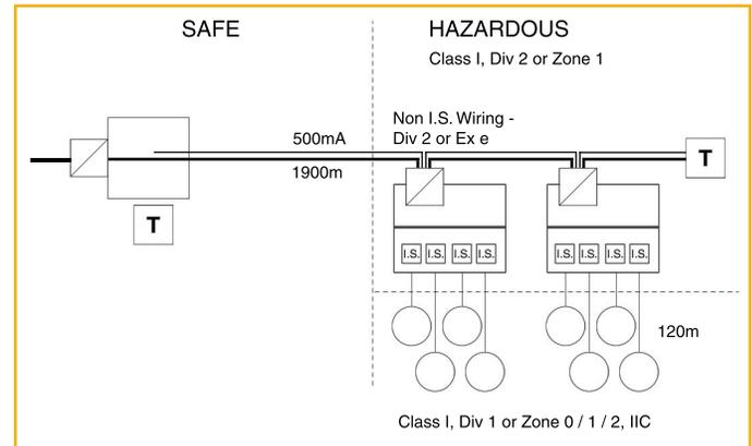
9 volts at the device, but 16 volts minimum at the field barrier. Furthermore, the field barrier itself is complex since the conversion from non-I.S. to I. S. must take place in the field barrier which is in the field enclosure. Since the enclosure uses both intrinsically-safe and non-intrinsically-safe wiring methods it can confuse field technicians and unfamiliar contractors.
