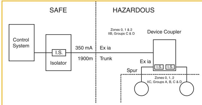
is sufficient for IIC Groups A, B, C & D. Since infallible resistors are used, devices from Zone 0/1 or 2 can be direct connected.
