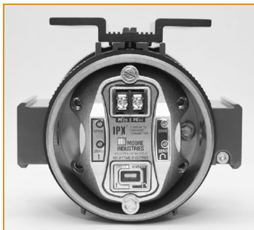
Figure 5. The IPX 2 is shown with the removable electronics module. This allows quick field replacement of electronics or removal when draining is required after liquid "slugs" appear in the air/gas supply of the unit. Replacement electronic modules are only available for IPX 2 units with S/Ns greater than 2321590.
